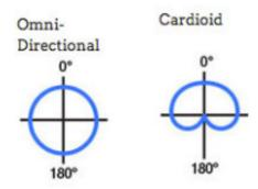
Figure 4: Microphone characteristics
